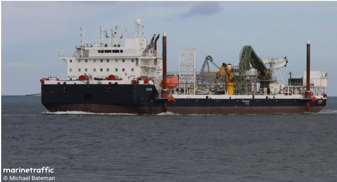
Figure 7: Cable Lay Barge ULISSE will be supporting cable landing and shallow water cable installation.
