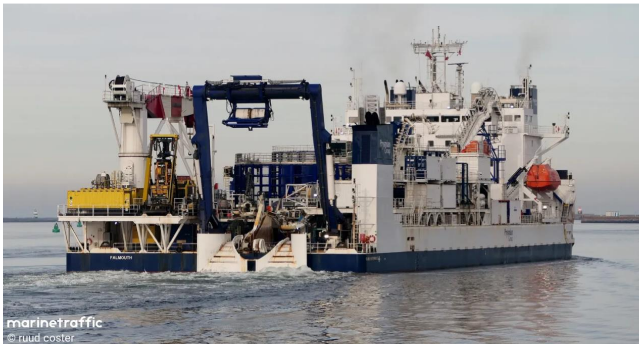
Figure 6: Cable Lay Vessel CABLE ENTERPRISE, with burial tool positioned on the stern, will conduct deep water cable installation.
