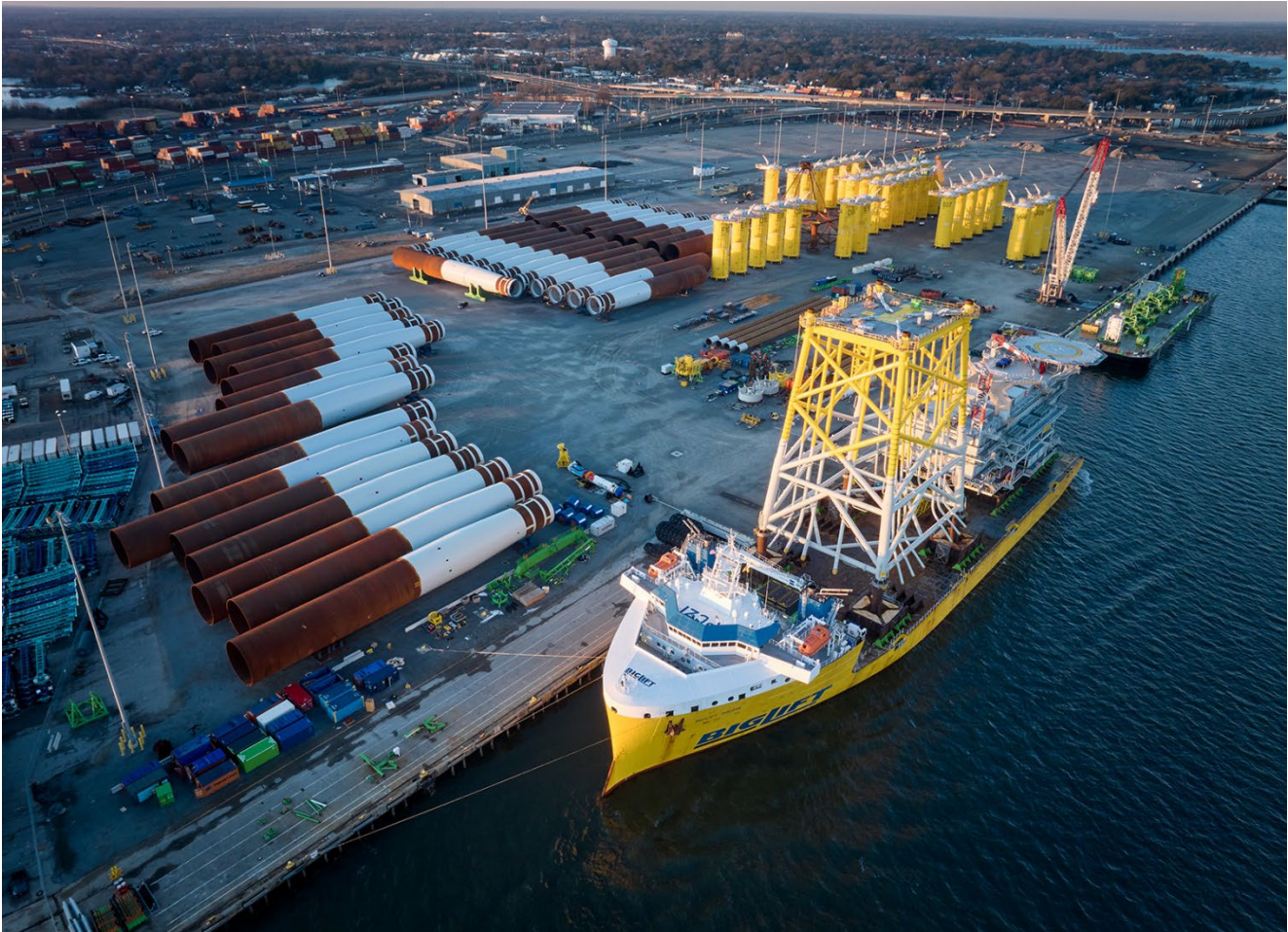
Figure 7: Offshore Substation topside and jacket arrival at Portsmouth Marine Terminal
