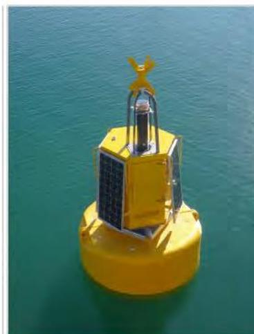
**Passive Acoustic Monitoring Buoy**
