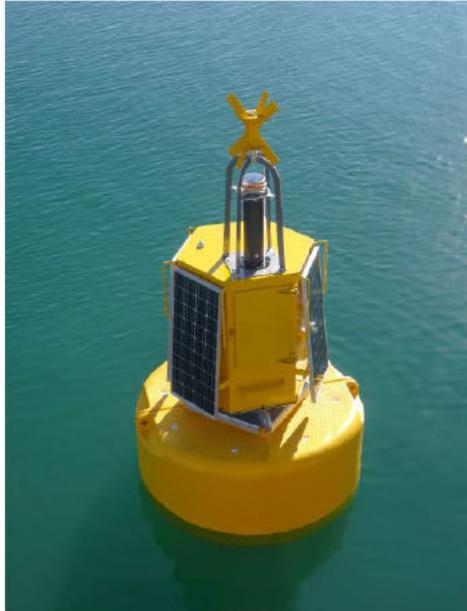
Figure 1: [REDACTED] AI acoustic monitoring and recording buoy
