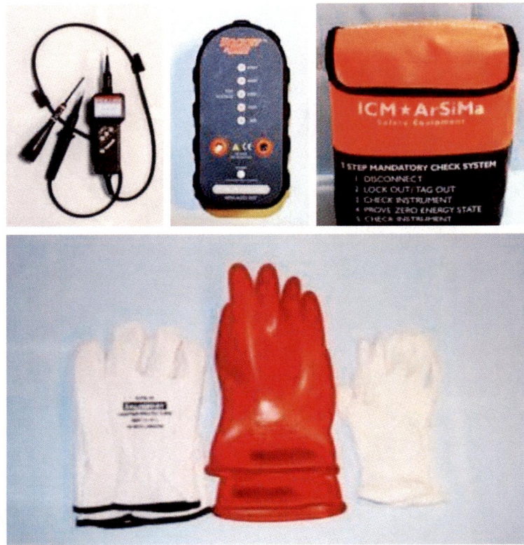
Figure 1: Sample photo of safety gear used for LOTO in Offshore Wind
