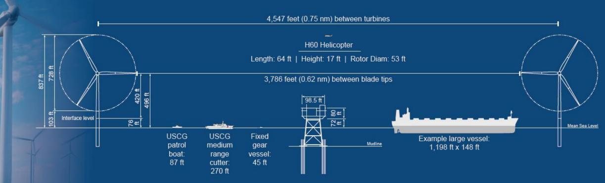
Depiction of different types and sizes of vessels and aircraft between two wind turbines, spaced 0.75 nm by 0.93 nm. These vessel and aircraft graphics have been drawn to scale to more accurately demonstrate transportation navigation and clearance between turbines.
