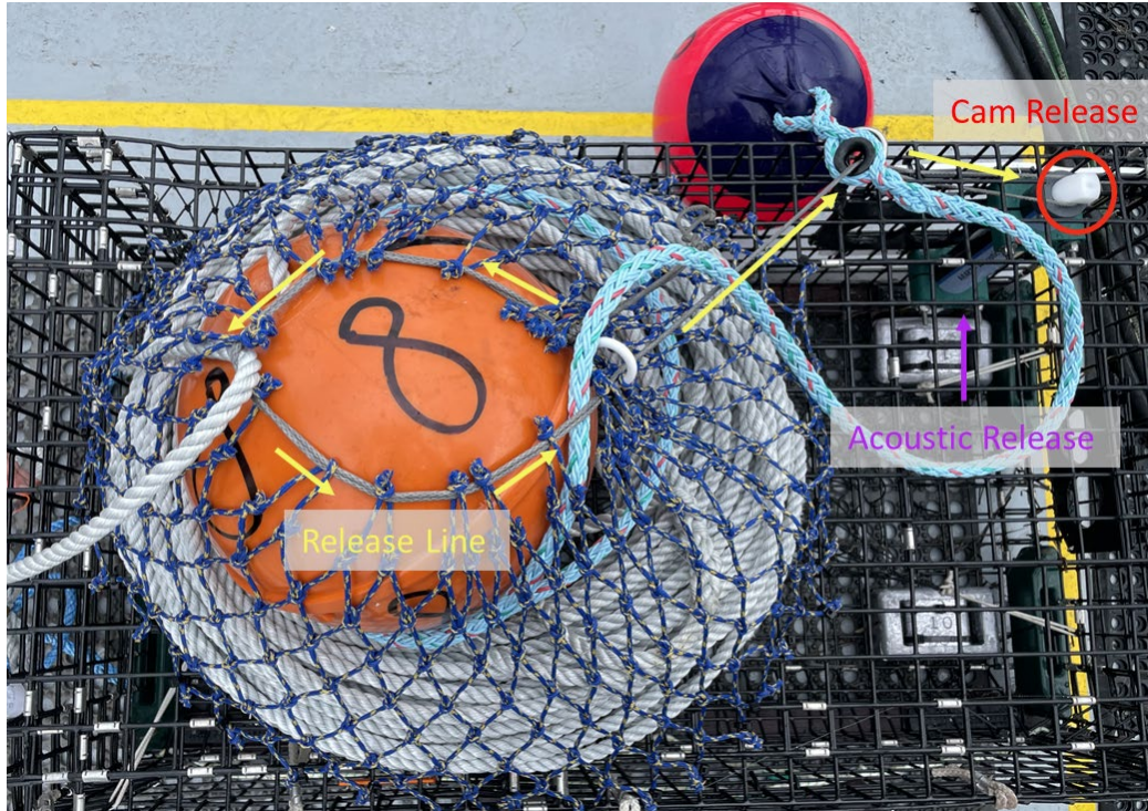
Figure 2. Image of the Guardian Ropeless System and acoustic release (purple) attached to a black sea bass pot and set for deployment. The release line (yellow) runs through the net and wraps around the cam release (red) holding down the buoy line and float.
