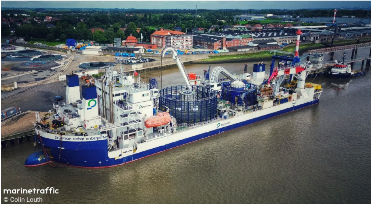
Figure 6: Cable Lay Barge CABLE ENTERPRISE will be supporting cable landing and shallow water cable installation
