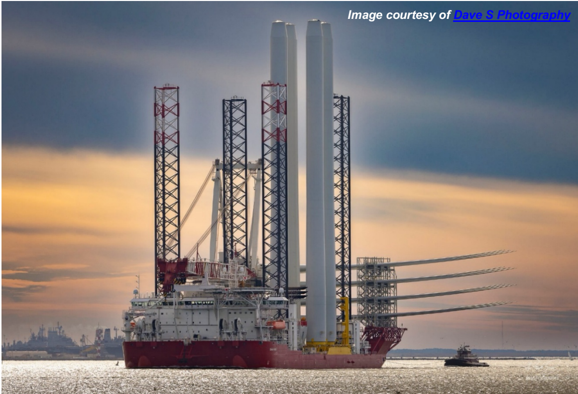
Figure 4: WTIV CHARYBDIS loaded with materials to support installation of four (4) WTGs in the Lease Area
