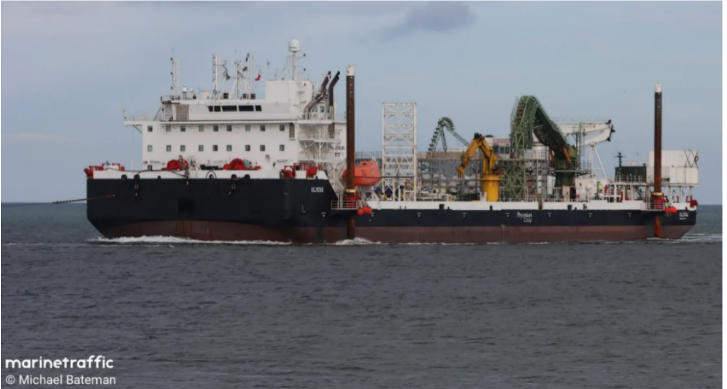
Figure 8: Cable Lay Barge ULISSE will be supporting cable landing and shallow water cable installation.
