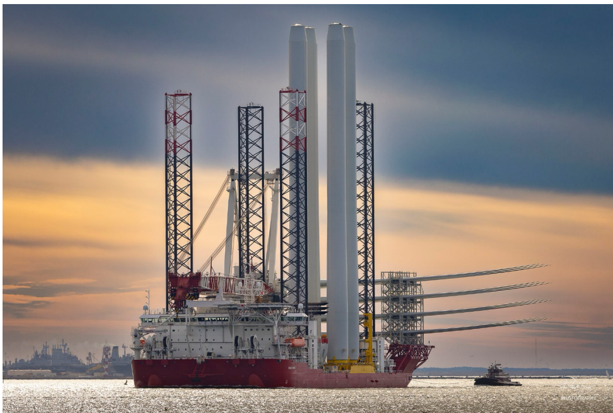
Figure 4: WTIV CHARYBDIS will perform WTG installations in the Lease Area.
