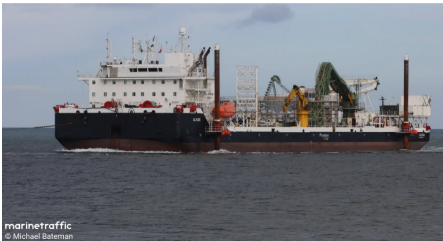
Figure 8: Cable Lay Barge ULISSE will be supporting cable landing and shallow water cable installation.
