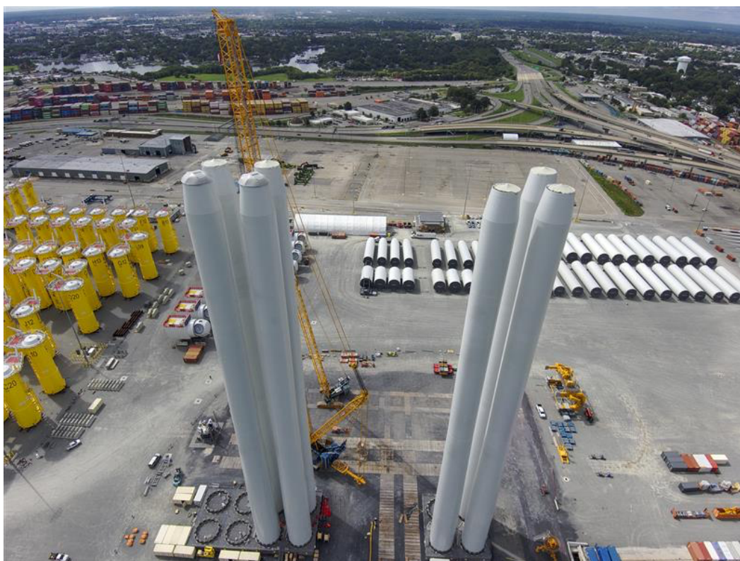
Figure 12: Completed Towers Quayside at Portsmouth Marine Terminal
