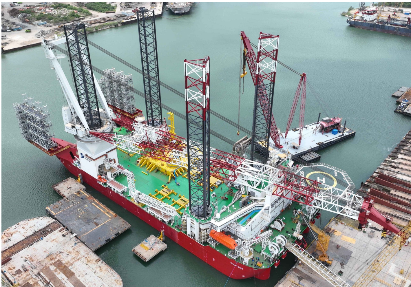
Figure 7: WTIV CHARYBDIS will perform WTG installations in the lease area.
