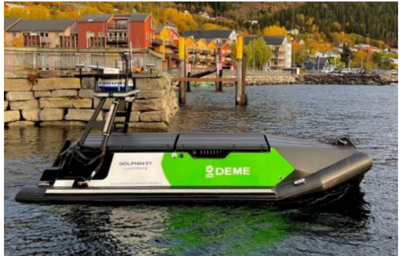
Figure 5: Uncrewed Surface Vessel (USV) DOLPHIN01
