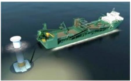
Example of fall pipe vessel installing scour protection
