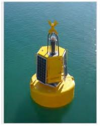
**Passive Acoustic Monitoring Buoy**
